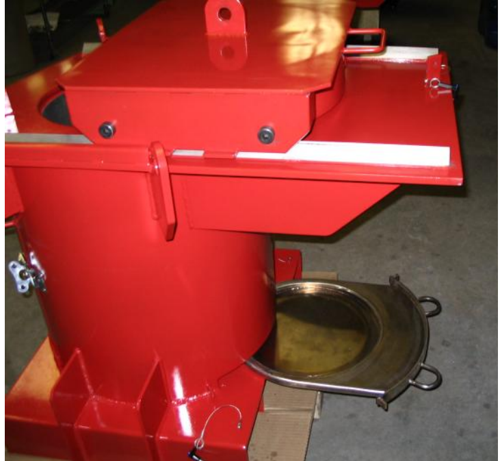
Filter Characterization Shield. Cover shown partly retracted drip pan shown retracted.
