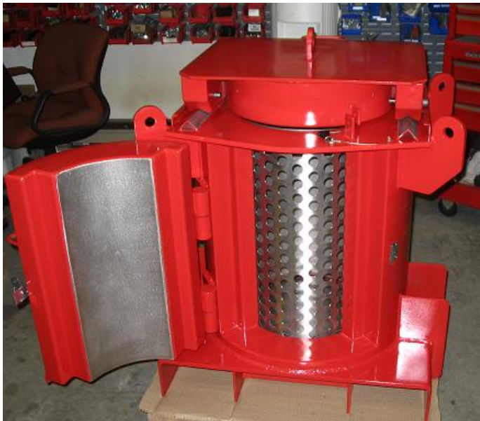
Filter Characterization Shield. Door opened, retention grid in place. S/S interior and enamel painted exterior.
