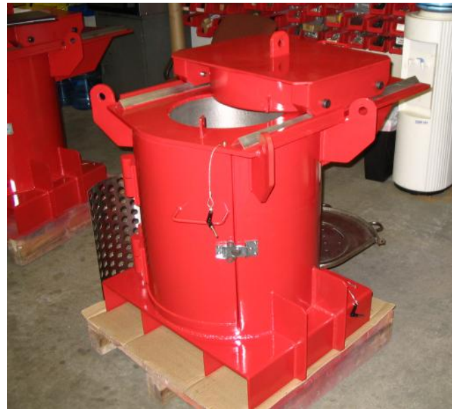
Filter Characterization Shield. Door closed, cover partly retracted.
