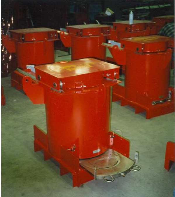
Filter Transfer Shields. Foreground, drip pan shown retracted.
