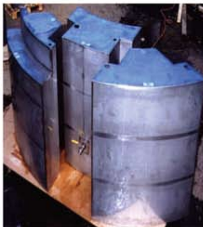
Shown below: Stainless steel, modular, water, Reactor Head Stand Shields featuring a stepped interface between segments to eliminate streaming.
