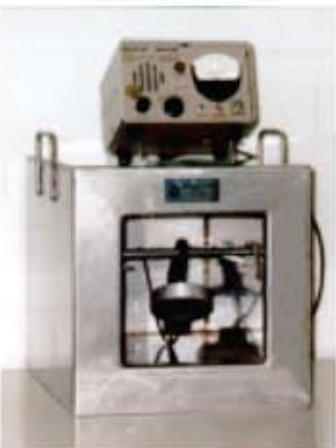
Shown above, left: FC-2 Model Frisker Cave with RM-14 Radiation Monitor. Shown above, right: Reactor Head Stand Shield installed on site, constructed of lead encased in steel. Typically, Reactor Head Stand Shields consist of 4 to 6 segments and outside diameters range from 13'-0" to 14'-4".
