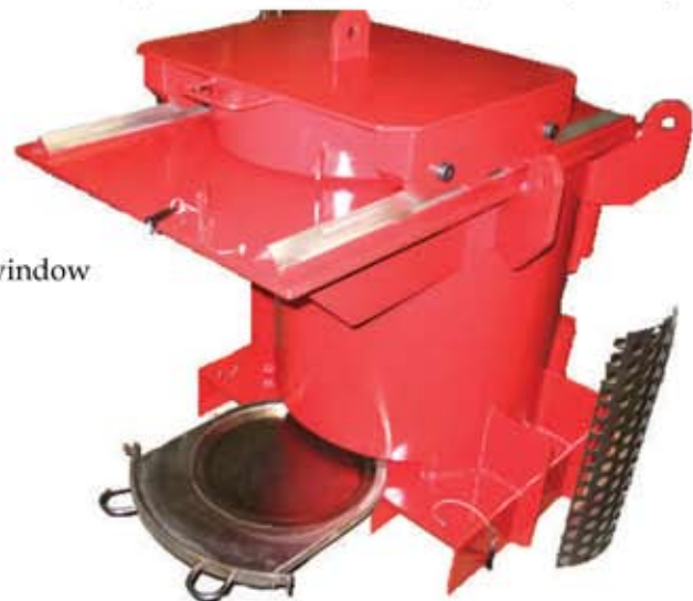
Shown above, right: A Spent Filter Shield equipped with a sliding lid and lockable stainless steel drip pan. Four V-groove wheels roll along stainless steel tracks to retract the cover.
