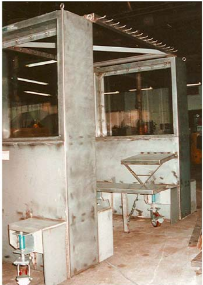
Two Window Water Shields connected with Blanket racks. Units shown have spring loaded casters.
